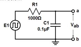
E1 is a voltage source that generates a square wave. Calculate its period, T, so that it is "high" for  $5\tau$  and "low" for  $5\tau$ . This period will insure that the voltage,  $V_{ab}$ , will stabilize to the voltage on E1 before each transition. Find the frequency, f, by computing f = 1/T.
